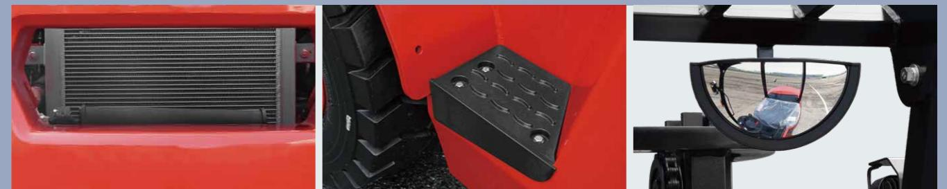
1. The radiator adopts aluminous plate-fin radiator with better performance and higher structural strength. Impendent oil radiator, optimized oil and water heat dissipation channel and double ventilation holes on counterweight can greatly improve cooling efficiency and reliability of overloaded operation and ensure reliable operation of the engine.
